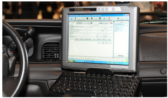
CIS' active Mobile Computer System (MCS) in the Rosemont Public Safety squad car at the 2011 IACP Conference. The MCS is a direct link between dispatchers and officers on patrol.
