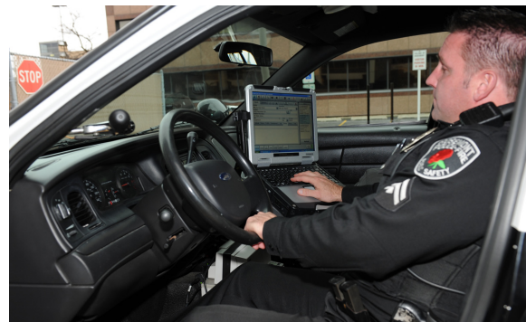
Public Safety Officer Michael O'Neill views an incident report on CIS' Mobile Computer System (MCS). MCS allows officers to see active incidents, while providing full access to all records in the main CIS database and running LEADS transactions while in the field.
